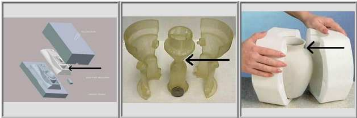
Figure 2: The casting direction is the direction of the cast removal. All of the objects have undercut features (pointed by the arrows) that prevent the direction perpendicular to the cast removal direction to be castable direction.
